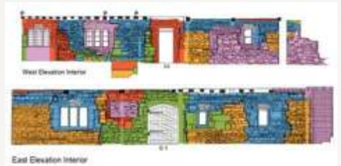
Interior recording elevations of the late-medieval range's ground floor showing the various phases of alteration and repair
