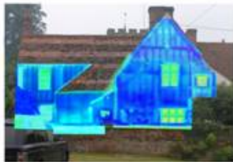
Fourteen thermographic images have been etched together and overlaid on the photo. The close-studded timber frame is clearly defined.
