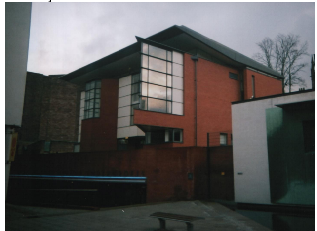
Youell House, seen from Priory Place. 'Letter box' window overlooking Cathedral Undercroft to the bottom left. Centre, acute-angled triangular oriel window.
